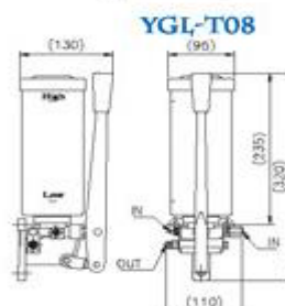
Pressure release device
